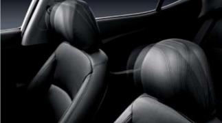
Front active headrests Front active headrests move forwards and up in the event of a rear-end collision to protect the head and neck.
