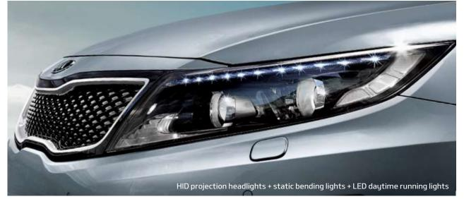
Optima's state-of-the-art lighting systems have been upgraded with surface-emitting LED tail lights, jewel-like 4-point LED fog lamps and LED daytime running lights integrated into the headlamp housing for maximum dynamic appeal.
